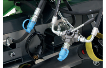
Sağ-Sol Kontrollü Hidrolik Vana Right-Left Controlled Hydraulic Valve
