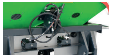
Sağ-Sol Kontrollü Hidrolik Vana Right-Left Controlled Hydraulic Valve
